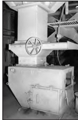
An installed SFD-2 in a coal-fired power plant provides an alarm output when there is an interruption in coal supply.
