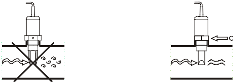
For pipe mounting, fork-tines must be parallel to the direction of flow
