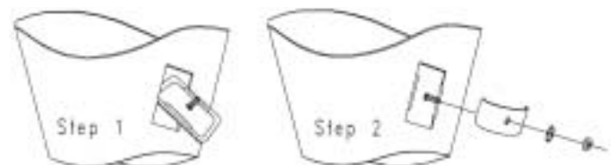
Figure 3B - Insert subassembly into vessel opening and secure subassembly to vessel with spring bracket. Secure bracket with hardware.
